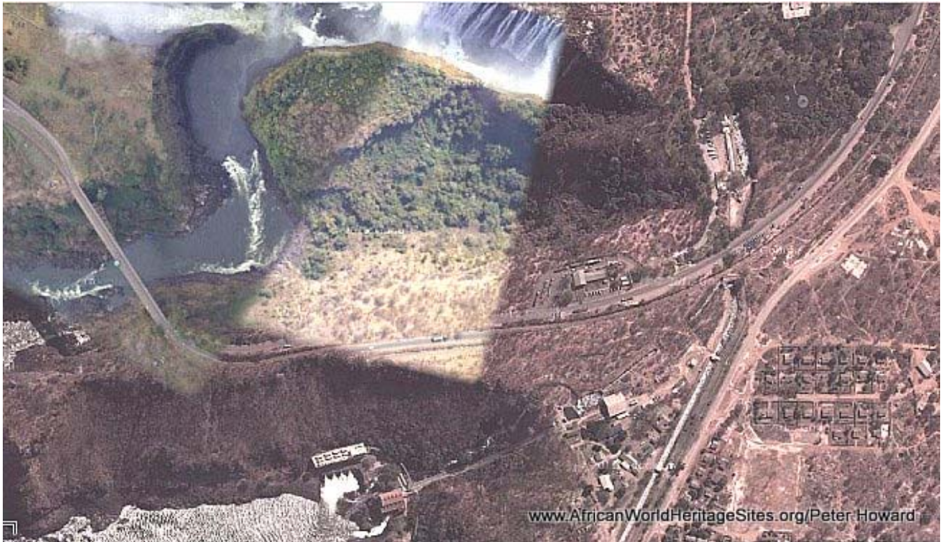
Satellite image of the eastern end of Victoria Falls showing the hydro-electric power generation facility which uses about half the dry-season water flow in the Zambezi River, diverting it away from the falls (Photo courtesy of Google Earth)
